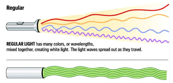
**LASER LIGHT** is of the same wavelength, with all of the waves in phase, or in step, with one another. A laser is always a single color because the waves are the same length. Because the waves are parallel, a laser light stays in a tight beam for long distances.
