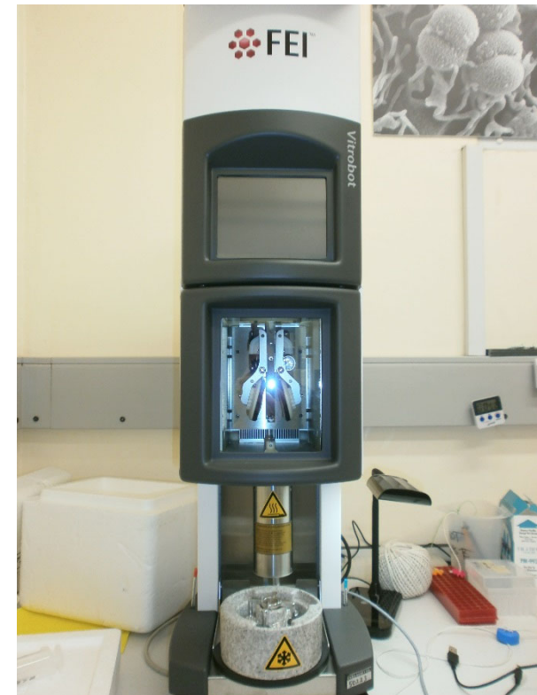
FEI Vitrobot for automated plunge freezing of grids
