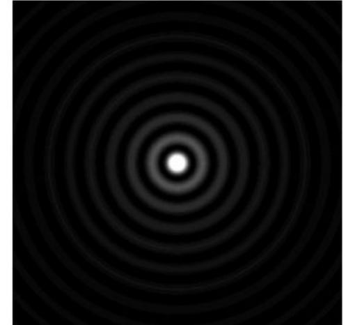
Core of a Bessel beam with light rings of equal energy surrounding it
