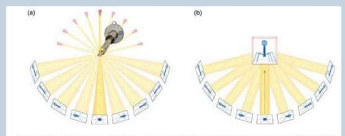
Principles of Electron Tomography. (a) A biological specimen, in this case a bacteriophage contained in an EM sample holder, can be imaged from several orientations by tilting the holder in the electron microscope. (b) Process of computed backprojection, in which each tilted view is used to reconstruct to three-dimensional information of the original structure. [McIntosh, et al. (2005) Trends Cell Biol. 15:43-51].
