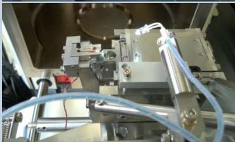
3. Block moves up 50 nm and the diamond cuts the surface
