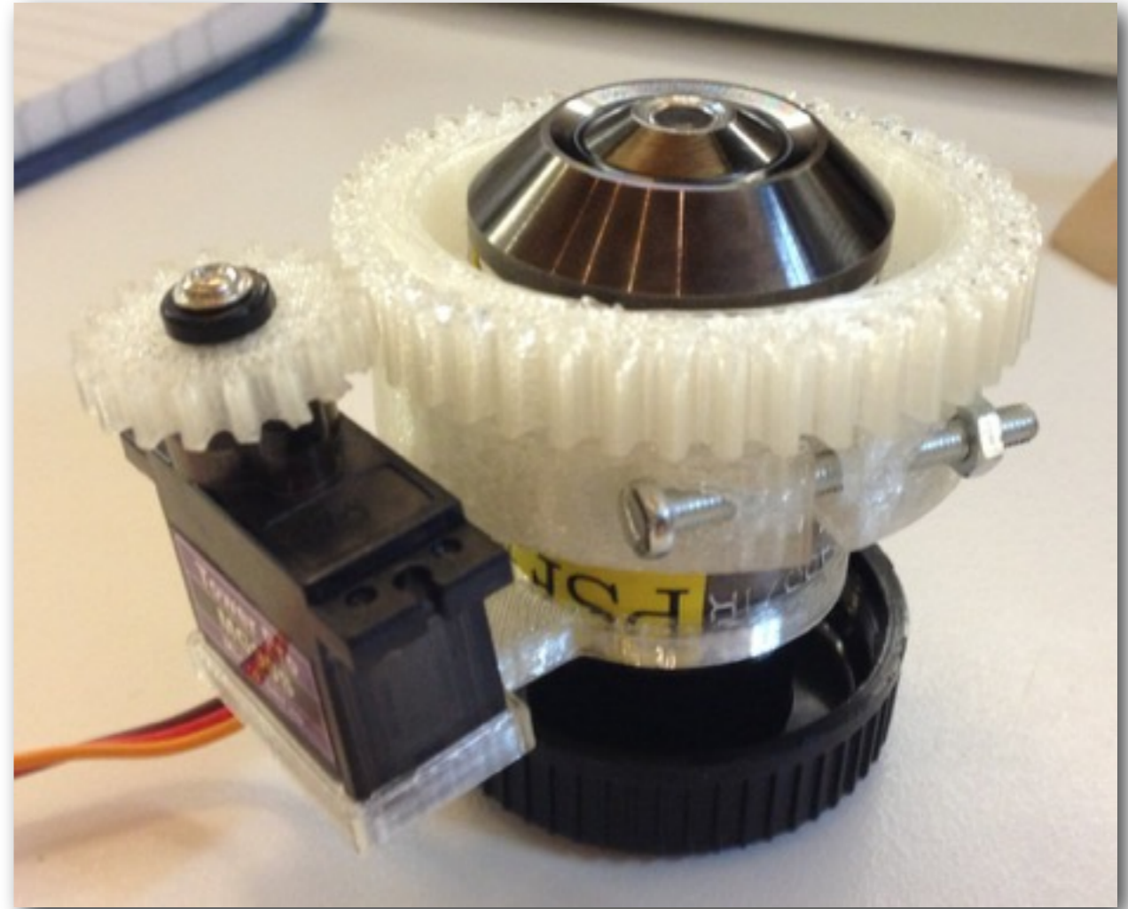
Jonathan Sturt, RMP: x60 SI lens - automated collar correction
