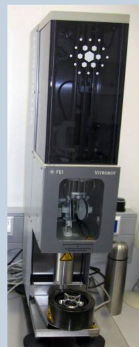
FEI Vitrobot for automated plunge freezing of grids
