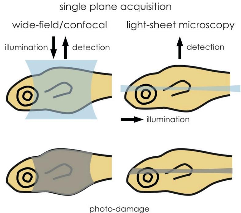
Compared with confocal and two-photon fluorescence microscopy, light-sheet exposes the embryo to at least three orders of magnitude less light energy, but still provides up to 50 times faster imaging speeds and a 10–100-fold higher signal-to-noise ratio.
