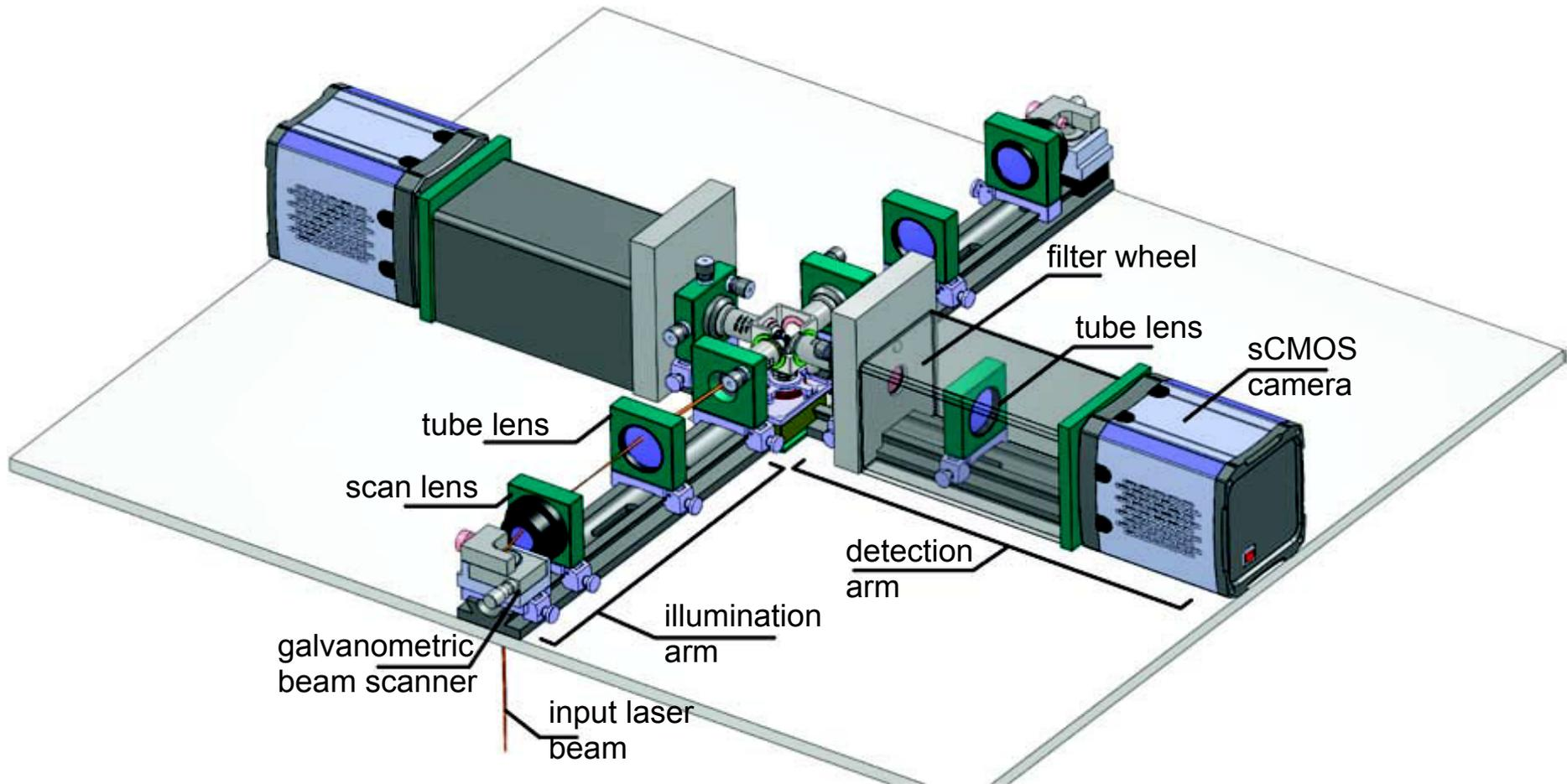
The two cameras simultaneously acquire stacks through the sample first with illumination by one light-sheet and then by the other thus eliminating the need for sample rotation and increasing acquisition speed.
