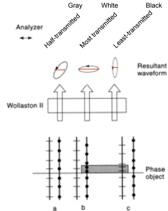
With bias retardation there is a systematic phase difference introduced by Wollaston II, such that light in "a" is already elliptically polarized. Now the difference between "b" and "c" is detected by the analyzer.
