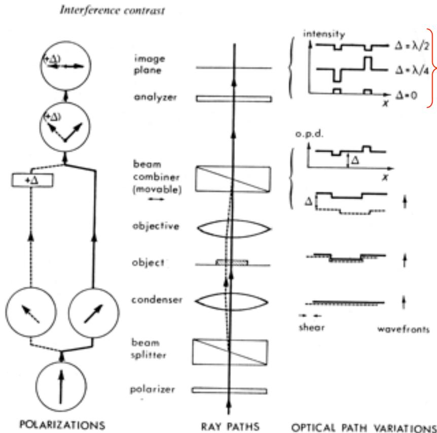
Fig. 38. The optical system for interference contrast.
